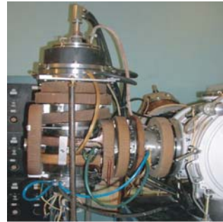
Fig. 1. T-shaped filtered vacuum-arc plasma source for diamond-like coating (DLC) deposition. Coating deposition rate is 6 μm/h at the diameter 20 cm
