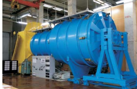
Fig. 2. General view of the stand-facility for thermo-vacuum testing of Space-vehicles
